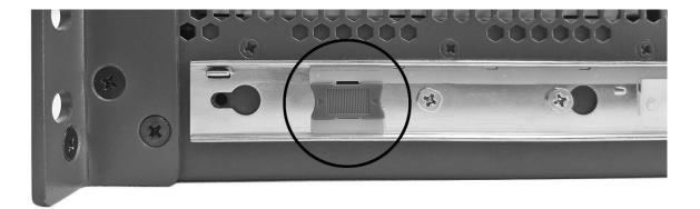
e. To lock the chassis into the rack, place a 5mm x 9mm screw through the bottom hole of the ear and secure it to the rail.
